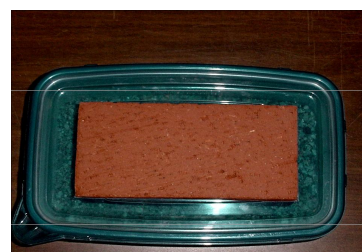
Container Set Up-Efflorescence Test
