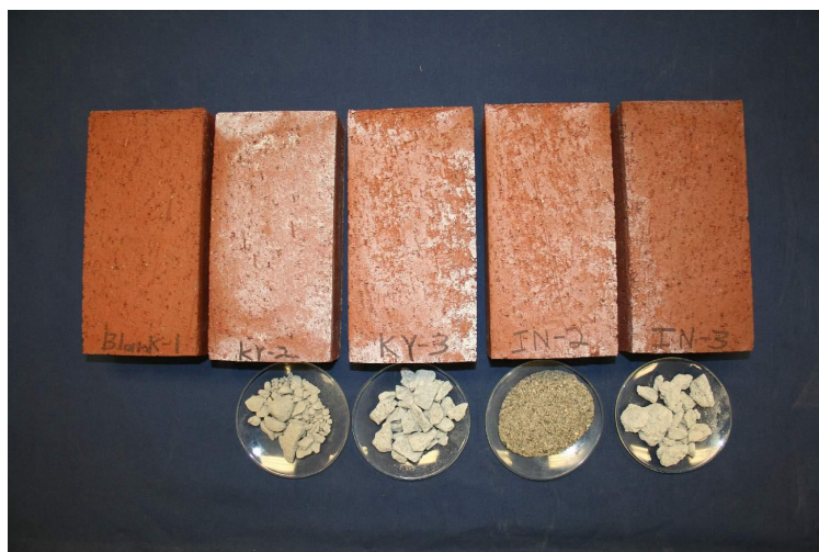
Aggregate Efflorescence Test Results (standard sample far left)
